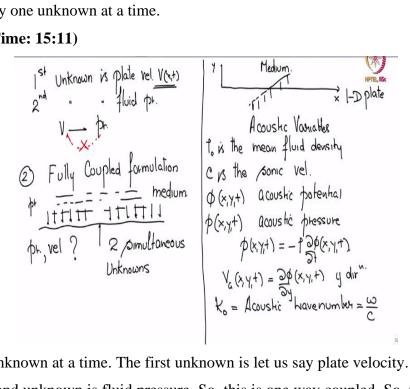
There is one unknown at a time. The first unknown is let us say plate velocity. Then after it is found, the second unknown is fluid pressure. So, this is one way coupled. So, why is it called one way coupled because in this case the velocity that you have found does not change anymore. The velocity decides the pressure. The pressure in turn does not or cannot decide or modify the original pressure, no that does not happen.
