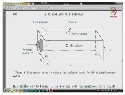
So, there is this box now, top cover is flexible, vibrates, other walls are rigid and it can be driven by a point force using an electromagnetic shaker and this wall can be; there is a speaker mounted that can drive the acoustic space. So,  $L_1$ ,  $L_2$  and  $L_3$  are the dimensions.
