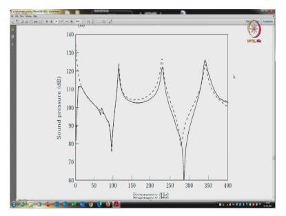
This is the sound pressure inside for experimental acoustic excitation a acoustic response with lymph masses placed on plate. A rigid, bald condition was assumed in the simulations b acoustic masses removed from the plate full coupled coupling was assumed in the simulations. So, this is the coupled response due to acoustic excitation and again these peaks, you see, are all the original resonances of the system.
