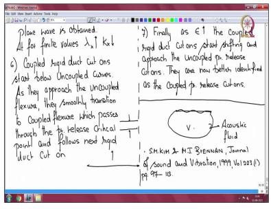
At infinite inertia the uncoupled plane wave is obtained couple plane wave is obtained and for finite values  $\lambda_x$  has to go up reduction of inertia and therefore  $k_x$  will start going down. I think point number six. The coupled rigid duct cut ons start below uncoupled curves as they approach the uncoupled flexure, they smoothly transition to coupled flexure which passes through the pressure release point pressure release critical point and follows next rigid duct cut on.
