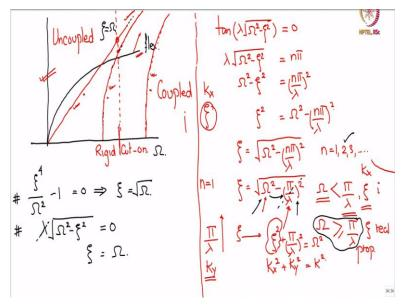
But further to this let us see on a diagram what these are so let me take an axis this is the nondimensional frequency axis. So let us look at  $\frac{\xi^4}{\Omega^2} - 1 = 0$  which implies that  $\xi$  is equal to  $\sqrt{\omega}$ . So, this is the non-dimensional flexural wave in the plate. So, it will look like this, so this is the flexure next we have  $\lambda \sqrt{\Omega^2 - \xi^2}$  when that is equal to 0.
