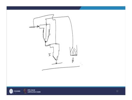
So, that is stage one. This is a cyclone. So, stage one raw coal is they will enter from here raw coal will enter from this side. High density due to centrifugal force high density for particles will stick to the surroundings and it they will drain down right and the low density particles they will go up with the swirl and leave the cyclone. No they will leave the cyclone and they will be collected somewhere else.
