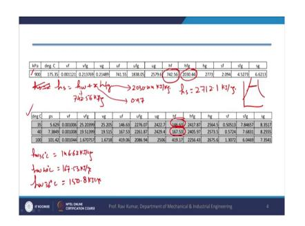
So, now here we will look at the properties of a steam will take the steam table. So, hs that is enthalpy of saturated water enthalpy of saturated water at 9 bar and that 9 bar because here the vapor is not superheated right it is 0.97 dry. So, if we draw the temperature entropy diagram so, the heating is terminated here. It does not go up to the saturation level.
