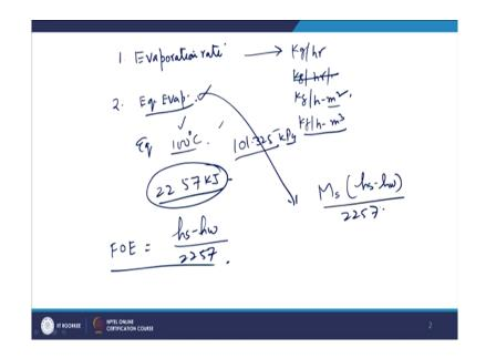
Now, the first parameter is evaporation rate. How much water is getting converted into this? So, there are certain units for evaporation rates for example, this is kg per hour. Now, kg per hour per meter square, kg per hour per meter square; because there are different boilers having different combustion area right. So, if the boiler is larger in size definitely it will producing more steam.
