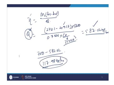
Now, efficiency is equal to mass steam hs minus hw divided by heat supplied. Now we have efficiency with us. We can always calculate the heat supplied.
