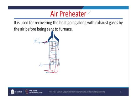
So, a typical arrangement of this the vertical tubes, bunch of vertical tubes and where the hot gases are flowing in this tubes, hot gases are flowing through these tubes, right. So, they are vertical tubes hot gases are and they are leaving here from the top, right. And cold gases are entering from this side.
