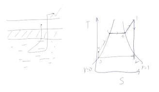
If you look at again Rankine cycle, right, and a temperature and trophy diagram X is equal to 0, X is equal to 1. So, this process 1 to 2 takes place in a turbine and not this is not like that
