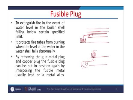
So, let us start with a boiler mountings. There is a fusible plug which is required in almost all fire tube boilers. If fire tube boiler is a boiler, where in the shell the water is filled and there is a tube that maybe 1 tube or maybe 2 tubes or 3 tubes which are carrying the hot fuel gases which are burned in the combustion chamber of the boiler and these hot gases are surrounding by the water.
