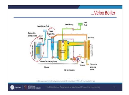
Now, this is the arrangement of Velox boiler. Here combustion chamber is shown. This is super heater, this is turbine compressor which supplies air for burning the fuel, then number of tubes you can see here and there is the steam separator. This is an economizer and this is the entire arrangement for the Velox boiler.
