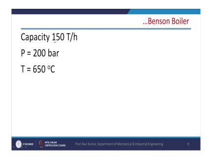
The capacity of Benson boiler is 150 tons per hour, pressure is 200 bars quite high and temperature also we can attain 650 degree centigrade.
