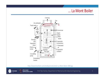
So, this is the arrangement of a La Mont boiler. This is the schematic arrangement which I have explained you here, they have put the air pump here. Again it is a u type of I have put air pump here. It does not make any difference and air is used for preheating ok. After the La Mont boiler, we will take up Benson boiler.
