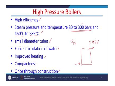
So, the green boilers, they have efficiency more than 98 percent and very low level of NOx solution to the surroundings. Regarding the pressure and temperature as I said earlier high pressure boilers have pressure more than 80 bar. So, the pressure varies from 80 to 300 bars and a temperature of steam 450 to 585 even it exceeds 600 degree centigrade. So, high pressure boilers have you can have the temperature of steam up to 600 degree centigrade, pressure up to 300 bars.
