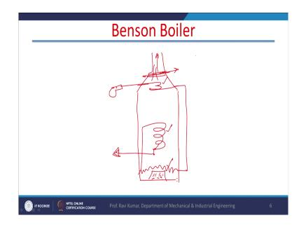
Now, Benson boiler is a drumless boiler it does not have any drum. So, it is a once through boiler. So, I will make the same type of schematic here also, there is a shell, there is a neck of the shell and then exhaust of the gasses right. It is a once through boiler. So, feed water feed water will be entering from the top because economizer has to be at the top economizer below that the convective heating, below that radiation heating.
