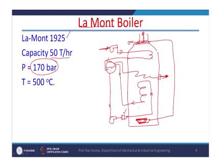
So, the most popular boiler is La Mont boiler which was introduced in 1925. The steam generation capacity of La Mont boiler is 15 tons per hour, pressure is 170 bar and temperature it can it take up to 500 degree centigrade. In a La Mont boiler, there is a boiler shell right and it narrows down from the top and this is the place for flue gas to leave the boiler. And, fuel is burned at the bottom of the boiler in fire wait.
