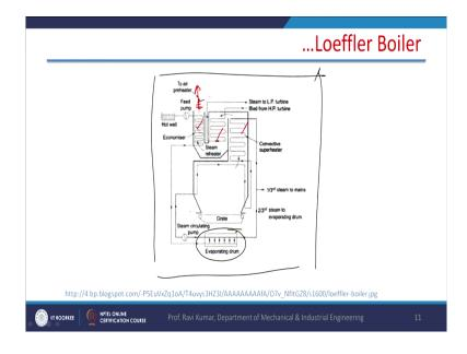
This is a schematic of this Loeffler boiler. Here you can see that this is grate, this is evaporated drum, this is super heater and here it is reheater for the purpose of reheating steam and this is economizer and from here, air preheater is also provided because after economizer air preheater will also be provided to preheat the air to trap the maximum amount of heat from the boiler right.
