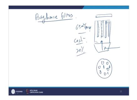
Another is bag house filter, in bag house filter the process is very simple in a box; in a box there are number of bags they are hanging from the header right and in the box the flue gas which enters from the bottom it comes into the contact with the bags and when this flue gas because they are connected at the same header top.
