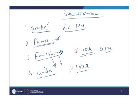
Now next is particulate emission. Now, this particular material you must have heard or you must have seen in the news also it is also quite damaging in for the health. And first of all is smoke, smoke which is coming out of the chimney it has particular material of diameter less than 10 micron, 10 micrometer. Very tiny particles are there in this smoke there are fumes which are also dangerous fumes may term from the coal or they come from the metal as well.
