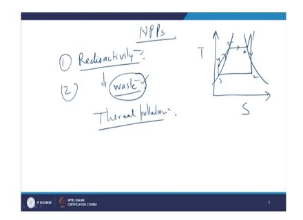
Another is nuclear power plants, in nuclear power plants there is no exhaust gas because the heat is generated if you look at the again Rankine cycle of power generation which is used for in a elastic super heat cycle. In a thermal power plant fossil fuel plant or in nuclear power plant the cycle is like this. So, this process 4 to 6 it takes place inside the boiler where the fossil fuel is burnt right.
