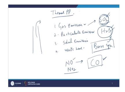
Now again in the thermal power plant, in a thermal power plant the pollution comes through chimney; main pollution comes through chimney right. And this emission which is coming out of the chimney can be classified as gas emission, then particulate emission as I told you earlier, then solid emission and 4 waste heat; I have already discuss with you.
