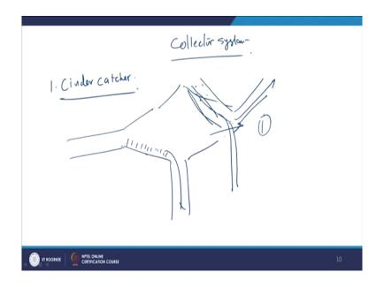
Now, collector system one is cinder catcher, right in cinder catcher what we do we use the second law of motion changing the direction of motion right. For example the cinder is coming with the gases in this direction you change direction of the motion. Because, they are solid nature it will go here and the gas will move from here.
