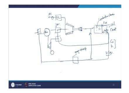
In open cycle MHD there is a MHD we can have an a schematic diagram there is a MHD it has magnets right. Just before MHD there is a nozzle, the function of the nozzle is it is a convergent divergent nozzle. The function of the nozzle is to provide the kinetic energy to the gases at the expense of pressure drop right.
