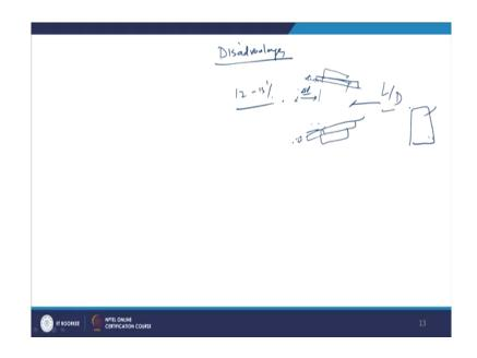
Disadvantages is when there is a flow of electron in MHD it is observed that this side becomes cooler and there is a reverse flow of electrons. Now, for in order to overcome this losses the L by D can be increased, or magnetic the length of the magnetic field is increased more than the required that is one thing. Or beyond the end of the MHD it can be extended. Friction losses
