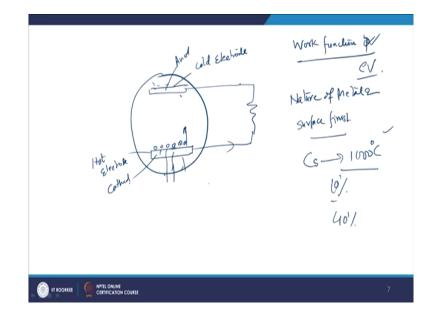
So, in a thermionic system, suppose we take a cylinder and there is a plate is a evacuated tube and this is cathode and cathode as coolant also. Because, due course of time this will get heated or its known as cold electrode right and this is hot electrode. So in fact, this is a cathode and this is this side is anode and this under vacuum this cathode is heated and electrons are liberated on from the surface.
