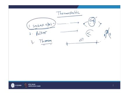
So, we will start with the thermoelectric conversion system thermoelectric, as it implies for the name itself thermo electric means heat into the electricity. Now, they are three effects one is Seebeck effect, another is Peltier effect and the third one is Thomson effect. Now, Seebeck effect says if there is a junction of the similar materials if there is junction of the similar materials right. And this junction these junctions are kept at different temperatures emf will be generated right.
