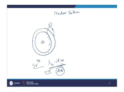
The last one is nuclear batteries the concept of nuclear batteries is that you take one shell and surrounded by another shell. And this shell is kept at low temperature by circulating a coolant right. Now, in the centre of this shell if you put some radioactive material the best suit age is strontium 90. The half life of strontium 90 is 28 years right.
