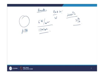
Now, so the anode should have a low for work function it should be like, so that, so barium or its strontium is used for this purpose. Cathode should have high, so tungsten is used for this tungsten is used for this. So, if we go temperature around 2000 degree centigrade as I said earlier in this case of cesium in other material also the efficiency is approximately 35 percent. Now, this system can be use of any fuel because we need heat only.
