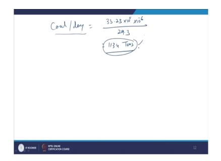
Now, coal required per day, total energy requirement 113.4 tons. So, you can compare the quantity of fuel required here, there only require 143 grams of uranium to produce the same power and for matching the power we need 113.4 tons of coal, right. That is all for today, right.
