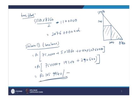
Similarly, for the base plant for the base plant, base plant we can find either we take area of this or area of this triangle minus area of this triangle. Area of this triangle we have already calculated. So, area of the bigger triangle is going to be 5000 multiplied by 8760 divided by 2 and it is going to be 114 minus sorry base plant minus this one, previous one, this, right and this will give us 2076 kilo Watt hour.
