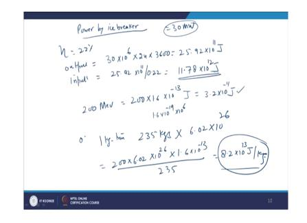
So, here power by ice breaker power by ice breaker, right is 30 megawatt, efficiency 22 percent. So, output is 30 megawatt, right into 24 into 3600 per day that is energy and it is going to be 25.92 into 10 to power 11 Joules.
