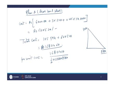
Now, cost of generation of plant B that is peak load plant, Plant A that is peak load plant. Now, for the peak load plant the cost is rupees plus 3 into maximum power generation capacity that is 1140 plus 0.015 into 114 and that is going to be equal to rupees 620520, right and for this one it was 1059940, right. So, total cost is going to be total cost, minimum cost is
