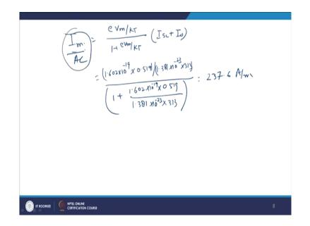
Now, after this V m is known now we have to find the value of I m, now, I m is equal to e V m by KT divided by 1 plus e V m by KT, I short circuit plus I o. Now, again we will keep on putting the values e is equal to 1.602 into 10 to power minus 19. Now, the value of V m is also known to a 0.519 divided by KT K is 1.381 into 10 to power minus 23 into 313, right divide by 1 plus again 1.602 into 10 to power minus 19 into 0.519 divided by 1.381 in to 10 to power minus 23 and T is 313, right.
