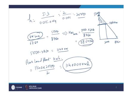
If you take h here in this case, then this is b 2 minus b 1, c 1 minus c 2. So, b 2 is b 2 is 5, b 1 is 3, c 1 is 0.015, c 1 is 0.015 and c 2 is 0.014, right. So, here h is equal to 5 minus 3 divide by 0.015 minus 0.014.
