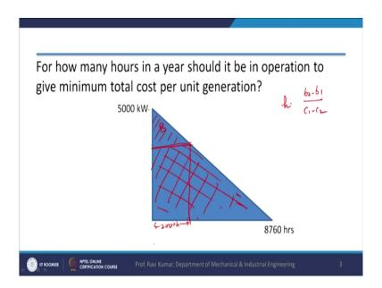
So, we have to decide this is a load curve is here, this is the load curve, this is a straight line, right. So, we have to take a combination suppose we take entire power 5000 kilo Watt from B, right. If we take entire 5000 kilo Watt from B this the fixed cost will increase, this capacity wise cost will be high.
