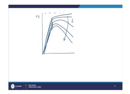
Now, suppose no not like this. Its curves are like this and we are getting maximum here. And for this maximum value, we have used this equation. We can have from if you look at this equation, we can have the maximum value of 16 by 27; 16 by 27 and this 16 by 27; the 16 by 27, it turn out to be 0.593.
