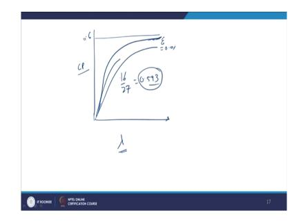
Now, if we take into the account, then and if you draw the graph between C p and tip speed ratio lambda and coefficient of power coefficient Cp; Cp is power coefficient and this is tip velocity ratio and this is 0.6, we get a graph like this. And when the value of drag coefficient epsilon, this is epsilon; now this is epsilon is equal to 0.01 and when epsilon keeps on increasing.
