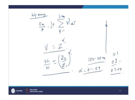
Now, hourly energy; hourly energy contains. So, E m divided by A is equal to half rho; i is equal to 1 and i is equal to hour is equal to v i cube delta t. So, this is hourly and if you want to do monthly, we simply take monthly data right. There is a power law also if we move to a height, the velocity will change right and there is a power law that is velocity is equal to Z raised to power alpha.
