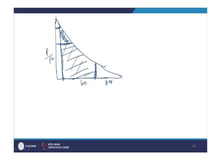
Now, let us go back to the design of a wind turbine because wind every power generating system has to be designed for a particular rpm and it is effective in a particular range only. So, if you take the cumulative frequency like this power density, power divided by density and this is hours and 8760 right.
