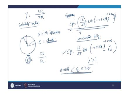
Now, there is a solid ratio also or solidity ratio not solidity ratio and solidity ratio is N C upon pi R. It is the ratio of the blade area, suppose in a turbine part of the circumferences plotted with the blades. So, it is the blade area and total frontal area that is known as a solidity ratio.
