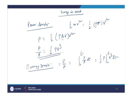
Now, energy in the wind, now energy in the wind, the one term is power density; power density. So, wind has kinetic energy that is half mv square and m dot is the mass flow rate. Now, if we take the mass flow rate, then half mass flow rate is the density into volumetric flow rate; volumetric flow rate V square v is the velocity; small v is the volume.
