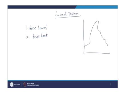
Now, load division, how we will share the load, load, load division between the power plants. So, there are two type of loads one is base load, another is peak load right. Suppose, month wise power consumption energy consumption is suppose is not like this. (Refer Slide Time: 05:36)
