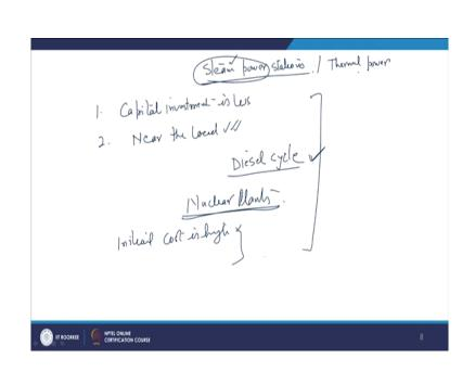
Steam power stations, now steam power station the best that is thermal power station, thermal power, steam or thermal power right, capital investment is less right, but operating cost is high right. So, capital investment is less, can be located near the load, steam power plant can be located near the load. There is no there are no issues only availability of coal is concerned and coal can be transferred transported by the railroad.
