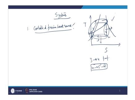
Now, nuclear power systems, what are the systems which are involved in the nuclear power plant, so it has to have controlled fission heat source fission heat source, because nuclear power plant also works from the Rankine cycle. If you look at the Rankine cycle on temperature-entropy diagram right, so 1 2 is expansion in the turbine, 2 3 condenser, and 2, this is 3, 3 to 1 4 1. So, process 3 to 4, 3 to 4, and this is 5, and this is 1.
