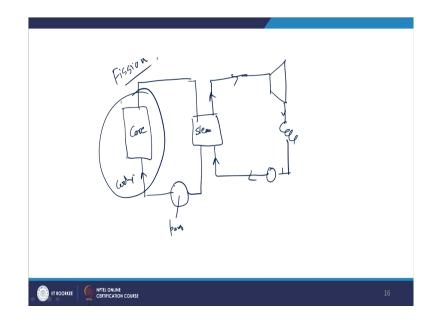
So, if we now take the main component in the nuclear power plant that is one is reactor core ok, and coolant is entering from here. There can be a pump or a pump house. And hot coolant is coming from here; here there is a steam generator we are known as headers also, in headers the steam is generated right. And here then this steam goes to a turbine as I explained earlier turbine to condenser and condensers back to the pump.
