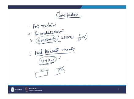
If you look at the classification; classification of a nuclear thermal power plant, so number 1 it is a fast reactor, another is intermediate reactor, and third one is slow reactor. In slow reactor also the neutron velocity is around 2100 meters per second or it carries the energy equal to 1 upon 40 electron volt.
