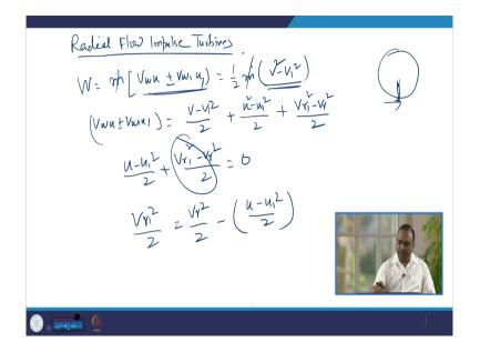
Radial flow means the, u keeps on changing right and u means the peripheral velocity of the wheel, it will keep on changing, as we move from inside to outside or outside to inside. Now the work output I have already explained it is mass low rate multiplied by Vwu plus Vw 1 u 1 it can be negative also so, plus minus Vw 1 u 1.
