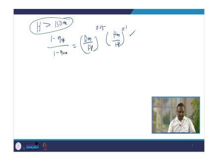
For head is greater than with the head is greater than 150 meters then mostly for the Pelton wheel or even Francis turbine also, this formula can be used when the head is greater than 150 meters that is all for today.
