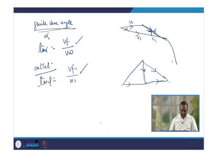
So, guide vane angle which is alpha can be taken as tan alpha is equal to Vf by Vw that can be taken from the inlet triangle because at inlet of the turbine this is this is the vane, this is Vr 1 r 1 and this is u and this is V 1 right and this is V 1 and this is alpha. So, guide vane will guide the jet in this direction V 1 direction wheel is moving with u direction and this will empower the relative velocity Vr 1 Vr in this direction Vr in this direction right.
