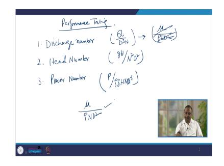
Now performance testing of turbines is very important, performance testing for the purpose of performance testing there are certain dimensionless numbers which are to be considered. For example, number 1 is discharged number it is Q by D cube N or Q by N D cube this is known as discharge number. So, if there is a prototype and the model right if in the model is same has to perform same as their discharged number should be equal.
