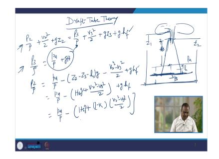
Now let us come to the draft tube, draft tube which I said is an integral almost integral part of any Francis turbine. Now what is draft tube theory, let us assume that there is a Francis turbine and fluid is moving after the radial moment it is moving in this direction and at the exit of the turbine there is a draft tube right. Draft tube is also submerged in water it is not left hanging otherwise the atmospheric pressure will come here.
