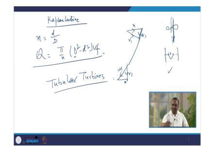
Now, we will discuss the Kaplan turbine, another reaction turbine is Kaplan turbine, Kaplan turbine is an axial turbine right. So, there is only axial there is sort of turbine blades are here
