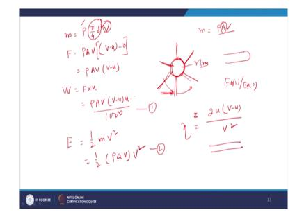
So, what is possible? The possible is if we take a shaft and we put a number of plates on the shaft. If you put number of plates in the shaft and if the water is strike the shaft here, right then
