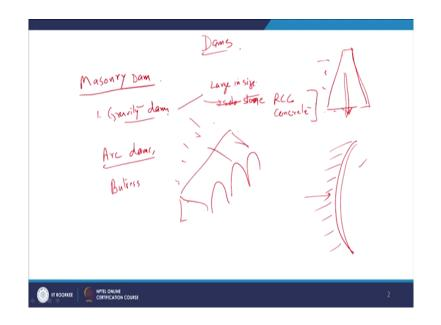
So, if you look at the Masonry dam. So, for example, Bhakra dam; Bhakra dam is a Masonry dam. So, one is gravity dam. Gravity dams are massive quite large in size and the thrust of the water because when the water is filled with the dam water on this side. So, thrust of the water is sustained by the gravity of ah this dam only, right.
