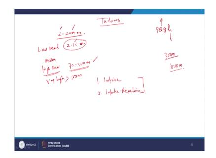
Now, we will go for the classification of turbines. Turbine is the main part of any hydro electric power plant because the power is produced inside the turbine, right. Now, turbine works between 2 to 2000 meter of head, there are turbines; there are turbines which are working under 2000 meter of head, there are turbines which can work up to 2 meters of head this is mini micro type of hydro power plant where they work for 5 meter head or 10 meter head or 7 meter head.
