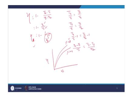
Now, here again I will write efficiency is equal to 1 minus T 4 minus T 1 divided by T 3 minus T 2. Now, here if you look at this is pressure ratio rp, rp is p 2 by p 1 is equal to T 2 by T 1 or we can say is raised to the power gamma over minus 1 over gamma is equal to T 2 by T 1. And in the same way it is T 3 by T 4, so here what we can do T 2 minus T 1 T 2 by T 1 is equal to T 3 by T 4.
