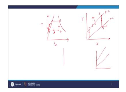
And we have amply discuss the Rankine cycle in previous lectures state 1 to 2 is expansion, 2 to 3 is condensation. Then 3 to 2 to 3 this is not 3, 4 is compression in the pump or pumping, and 4 to 1 the process takes place in the boiler. So, here all the processes they take place in a separate entities.
