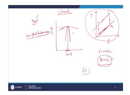
Now, we will discuss about the advantages of close cycles as I said earlier there are 2 types of gas turbine cycles; one is close cycle 1 is open cycle. So, if we compare the performance of a close cycle with an open cycle the close cycle has higher thermal efficiency, why? Because, if we again draw temperature entropy diagram T S state 1 to state 2, stare 3 to state 4 the entire this TS diagram can be shifted.
