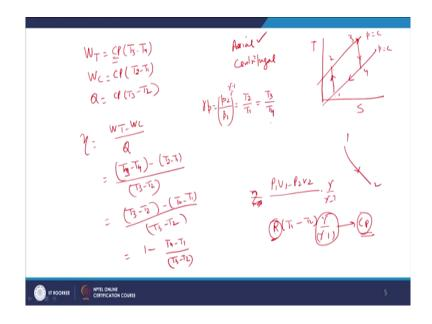
Now, if suppose we draw on temperature entropy diagram 1, 2, 3 and 4 right. So, work output work of the turbine is CP T 3 minus T 4; pressure is not constant it can always be asked, when pressure is not constant where you are taking CP. The reason being if you look at the work done in a adiabatic process suppose process is 1 to 2 right.
