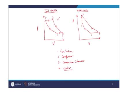
Now, if you draw PV diagram Joule cycle it will be more clear here, so Joule cycle will be something like this. This is the compression 1 to 2, process 2 to 3 is constant pressure heat addition, 3 to 4 is isentropic process where we gain the power output. And 4 to 1 when sub cooler is required otherwise this will go to the air.
