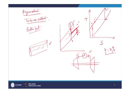
So, specific output of the turbine as i mentioned earlier it can be done by a regeneration, if the process of regeneration this is 1 to 2 right and 3 to 4. Now, exhaust is quite higher than the outlet of the compressor right, so with this exhaust this heated this is heated in a heat
