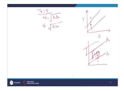
Now, efficiency can also be improved by reducing the compressor input, so this is state 1 to state 2. Now, for compressor input reduction, because we are dealing with air or gas which has a very low density in that case we can go for multi state compression. So, instead of compressing gas in 1 stage after compression in 1 stage the gas is taken away is state 1 this is state let us say 3, it is cool to state 4 and then again it is compressed to state 5.
