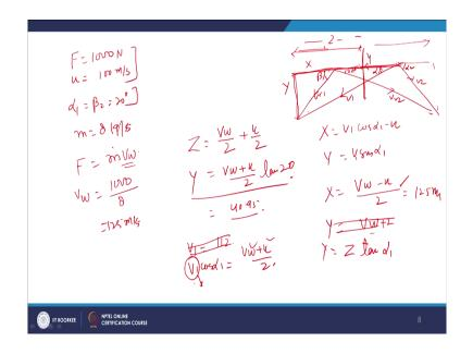
So, for this 4 sorry; so, for this the force is 1000 Newton right which is working on the blades and blade peripheral velocity is u is 100 meters per second. They are two things blade inlet; sorry nozzle inlet angle is equal to blade outlet angle 20 degree, they are all given values in numerical.
