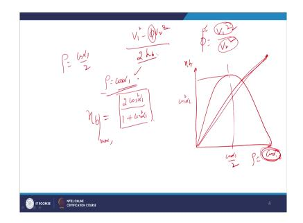
So, efficiency of the fixed blade when they are considered as a nozzle; efficiency of the fixed blade when they are considered as a nozzle is going to be V 1 square minus phi V 2 square divided by 2 h the blade, phi is carry over coefficient phi. Suppose because now what is happening fixed blade the steam is coming out with certain kinetic energy, but when it is entering the moving blade some losses are there.
