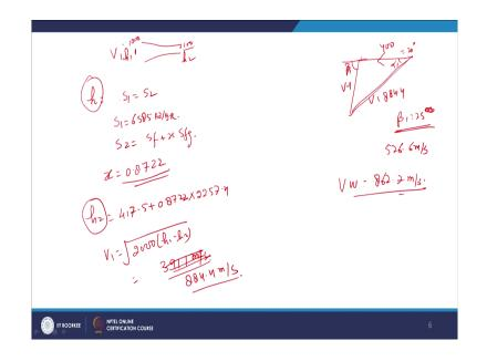
So, for that we will have to go for nozzle equations. So, nozzle up steam is 10 bar or 1000 kilo Pascal down steam is 100 kilo Pascal right. So, we will take h 1 here and h 2 here. So, h 1 is saturated steam at, saturated steam at 1000 kilo Pascal and that is 2777.1 right and because if we do not know the quality at the exit and quality at the throat as well right.
