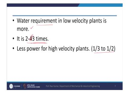
When the low the plant when the velocity is low in that case the water requirement is high. It is 4 to 2 to 4, 2 to 3 times, which is required for the mechanical handling system. So, in hydraulic handling system, it is 2 to 3 times and less power is required for high velocity plant. It is obviously 1 by 3 to 1 by 2.
