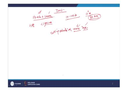
So, dust is they are in the power plant and this dust necessarily constitutes the fly ash plus smoke right. Now, they can be differentiated a smoke and fly ash can be differentiated through the particle sizes, the smoke particle is normally less than 1 micron.
