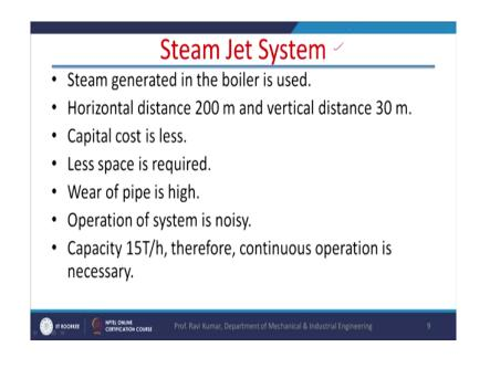
Now, the last one is the Steam Jet System. So, in the steam jet system first of all a steam has to be produced somewhere, if you want to use a steam. So, a boiler is used or steam generated in the boiler part of that steam can be used for the ash removal.
