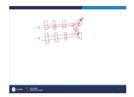
Now, there is a hydraulic handling system also. In hydraulic handling system, again there is a water turf, there is a water turf; and you can have number of water turfs and on each turf, the coal comes from the source right and water comes from this side. There is a force circulation right water comes from this side and there are sumps right and water is dumped into the sumps.
