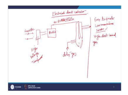
Now, in electrical dust collector, we take, we remove the dust particles by using high voltage. So, first of all three phase 440 volt current is used. This is supply and this 440 volt is converted into very high volt; very high volt means thousands of volts right. So, this is used by using high voltage transformer or this type of transformer.
