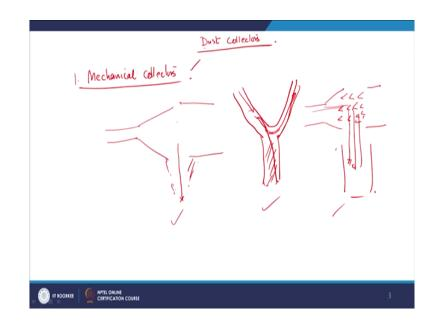
So, the easiest one is mechanical dust collector. Now, in mechanical collectors as it is clear from the name itself, they are devices which depend on the mechanical processes and here a typical mechanical dust collector will be something like this if you in a duct, if the dust is coming through it the dust is sucked through a duct right, and all of a sudden if you increase the cross section area.
