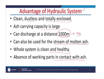
Especially the mechanical type of system it can remove 5 tons of ash per hour; that is a limitation of the mechanical type of ash handling system. But, there is and hydraulic system; let us talk about the hydraulic system, there are certain advantages of a hydraulic system. Hydraulic system, first of all it is clean; there is no dust, it is dust less, clean and the system is totally enclosed right.
