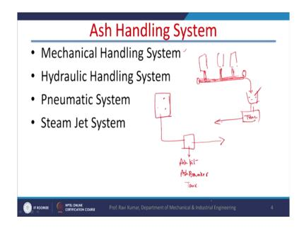
So, there are ash handling systems because, first of all, suppose there is boiler where the coal is burned. The coal is burned then, ash handling system will come into the picture through ash handling system, it will be transported to somewhere else. And, ash handling ash handling system it can be a mechanical system, it can be hydraulic system, it can be a numeric system or
