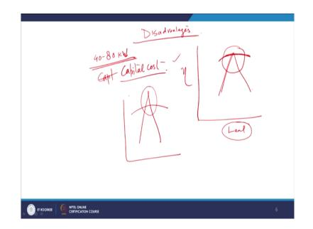
So, the disadvantages are: now disadvantages are: space requirement is more because, you need a transformer, a transformer followed by a rectifier, rectifier followed by the entire electrode systems. So, this occupies space and quite substantially spaces is occupied by the system and the system should be spark proof because voltage is very high; voltages of the order of 40 to 80 kilo volt.
