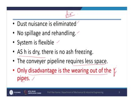
Here, the dust nuisance is eliminated. No spillage and re handling, system is flexible; ash is dry; there is no ash freezing; this is about the air system. Ash is dry in the air system right. The ash is dry; the conveyor piping requires less space because, air and ash these two things are to be handled right.
