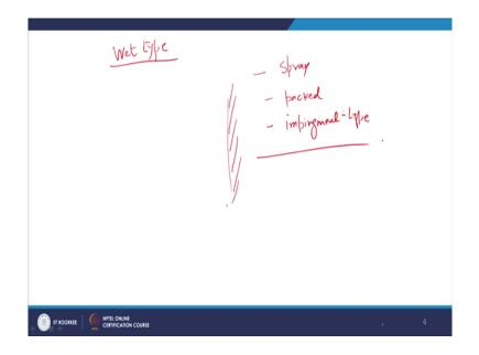
Because, particles if there is a wet cloth and if we pass the smoke to the wet cloth, number of the particles will stick to the wet clothes right. So, a wet surface is provided right and water is continuously sprayed on the wet surface and when the smoke is passed through this porous surface; porous wet surface, particles they stick on the surface. And when the particles it is just to ensure that the particles do not block the porous surface, continuous water is sprayed is made on the surface.
