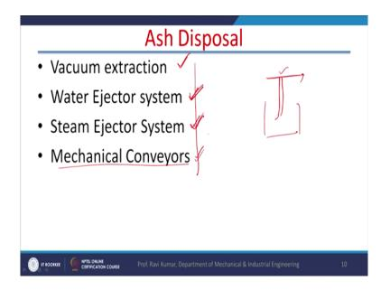
Now, ash disposal for the disposal of ash, there are 4 methods: one is vacuum extraction, water ejector system, steam ejector system, mechanical conveyors.
