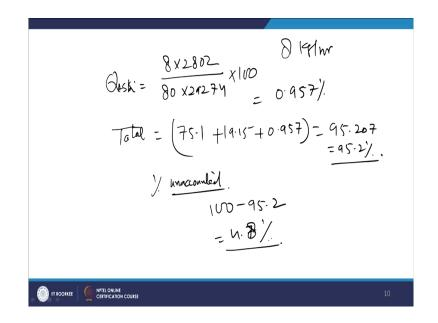
Now, mass of the air if you remember it is 8 kg per hour; this is the amount of ash which is being generated during the operation of the boiler. Therefore, percentage of heat because; calorific value of ash is given calorific value of ash is given 2802 Kilo Joules per kg and mass of the ash is 8 kg per hour right.
