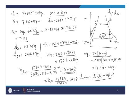
We will start with this, so first of all we will draw the Rankine cycle, ideal Rankine cycle or here in this Rankine cycle the steam is obviously, superheated. If you look at the steam table at this pressure of 140 bar and 550 degree centigrade, you will find that the steam is superheated. So, if you draw the Rankine cycle on temperature entropy diagram; this is X is equal to 1; the diagram is going to be like this. So, 1, 2, 3, 4 and this is 5 and the direction of the process is like this.
