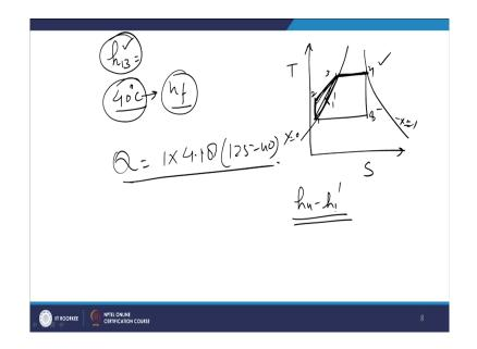
So, enthalpy first of all can calculate enthalpy at 13 bar; enthalpy of saturated vapour at 13 bar right.
