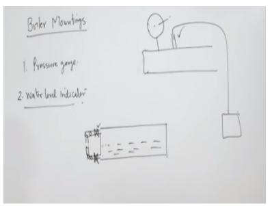
So first of all we will discuss about the boiler mountings now the first and fore most thing in the boiler is a pressure gauge because we must know what order of pressure is existing inside the boiler. So that boiler in a boiler the pressure gauge is fixed on the shell it is a dial type pressure gauge now a days digital pressure gauge is also available and pressure transmitter are also available and pressure transmitter are also available.
