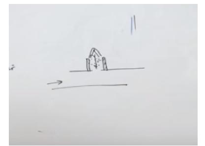
Now fusible plug very small in size and they are used in fire tube boiler and they are put on the surface of the fire tube right and this plugs have fusible materials we are filled with the fusible material means the major which melts in the high temperature right. So when the temperature exceeds from the certain limit the material filled in this fusible plug melts and water enters the grate and fire is extinguish and accident is prevented.
