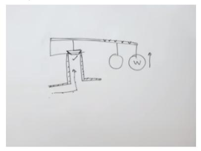
Level safety wall is almost like a diapered safety wall in this wall suppose there is a passage again and this side is fill with the team it as a lever that is why it is called as lever safety wall and this lever are on this lever arm on the extreme side there is a dead weight a lever safety wall. Now this dead weight it is edge here and this again is connected to a system which closes this open.
