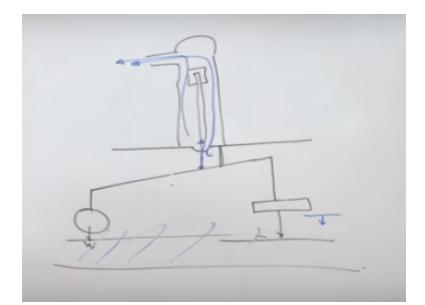
So in this type of wall there is a boiler shell wall of the boiler shell and there is opening this is semi-circular disk. It is connected it is exerting force on lever there is lever there is a counter weight W here there is float and it is reached here this lever is not end here it is changed here right. Above this again there is housing and provision for steam to vent.
