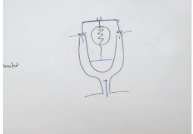
Here instead of putting weight if spring force is used for controlling the opening of the wall become in different shapes am taking a particular shape but they may come in different shapes this is a U type system on the both sides the valve is closed and steam is coming from this side. Steam I will show with glue pen so steam is coming from this side right and here there is a spring.
