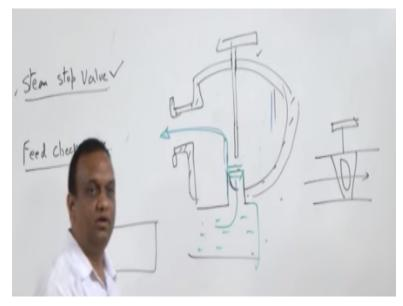
Steam stop wall is a normal valve to take steam out of the boiler as we have walls in the container to take water out of the container in similar fashion there is a steam stop wall which is connected on the boiler again there is a I mean this which closes this opening and this is of operated with a arm operated wheel right this is this keeps disk in the place this is the housing and from here we can get the steam.
