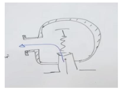
This is boiler shell this is opening this is stopper right above it there is a spring this is valve housing from here the exit of the steam is taking place they are flanges. So when the steam is exhaust the force on this stopper again it is lifted and steam is vented off through this opening. So there can be many arrangements so the working principle is the pressure of his steam is balanced with the help of tension in tension in the history.
