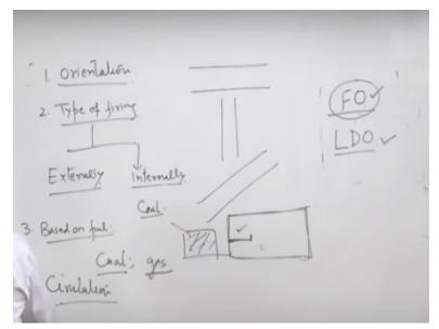
Orientation of vessel of the boiler right if it is if the vessel is horizontal it is over the horizontal boiler. If vessel is vertical it is vertical boiler if the vessel is inclined if it inclined boiler right. Type of firing it is firing of the flue. Now how the fuel is fired in some of the boiler or initially when the boiler were manufactured the firing was provided within the boiler some a great was provided now great the new term great.
