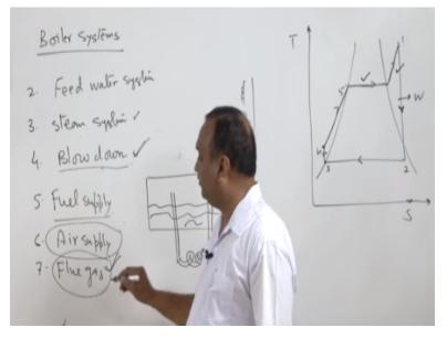
So regarding the boiler systems number one is water treatment system. Now water treatment system is we cannot use deaf water in the boiler because two TDS of deaf is water is quite high and it is not permissible to be used it is not permitted to be used in a boiler because when the water heating takes place in a boiler the solubility of salts in water reduces drastically.
