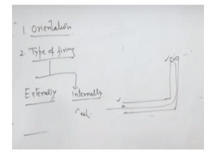
Suppose in a passage I have to circulate a air one method is I put a blower here and circulate the air in the passage that is known as force draft. Another way is I put a fan here or blower here which sucks the air through this passage it is known as induce draft. So either you go for induced draft in the boiler or force draft in the boiler or it can be a natural circulation.
