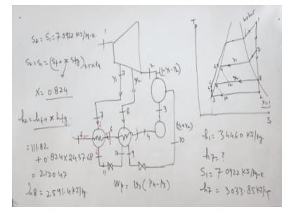
Suppose it is steam turbine steam will be tapped from various location and this steam will be used for heating the feed water going into the boiler. So first of all we will draw a temperature entropy diagram for the processes then physical we will draw the schematic diagram and then we solve it very well. Now this is temperature and entropy X = 0 and here X = 1.
