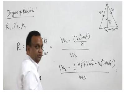
It is denoted by R, in some of the books it is denoted by Omega or capital Lambda. So the degree of reaction is again the temperature rise in rotor divided by temperature rise in stage or if you multiply by CP then energy imparted in rotor divided by energy imparted in stage or work in a stage or we can write work in a stage minus V two square minus V one square by two divided by work in a stage okay.
