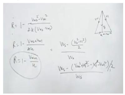
Now degree of reaction are is equal to, now instead of doing it here, we can write this is sorry V W two square + VF square - VF square. So this will be cancelled, so R is 1 - VW2 square - VW1 square divided by work in a stage. And the work in a stage is UVW 1 + V2 - VW1 VW2 - VW1 and this multiplied because this is 2 here this is divided by 2 and 2 will come here.
