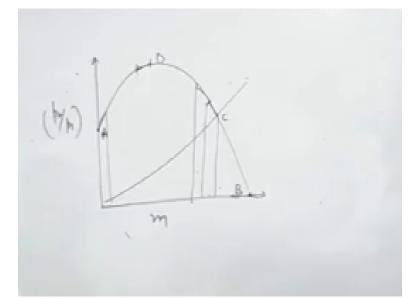
Now another phenomena is surging, let us draw the mass flow rate and pressure ratio and this is the surging curve. This is a characteristic curve and in this position there is a pressure ratio. But there is no mass flow rate it means the output valve is closed. Now in this position, mass flow rate is very high but pressure ratio is 0 it means the valve is fully opened, full throttle.
