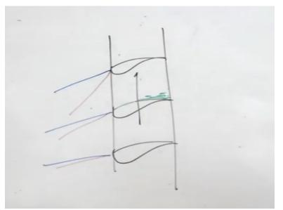
Suppose in a cascade there are number of blades let us take three blades and there is a different angle of incident changing and here at particular angle, the p and fag end he flow separation may take place. This is known as Stall and this is stall is not stationary it moves in opposite direction of the flow with half of the speed right and that is known as Rotating Stall.
