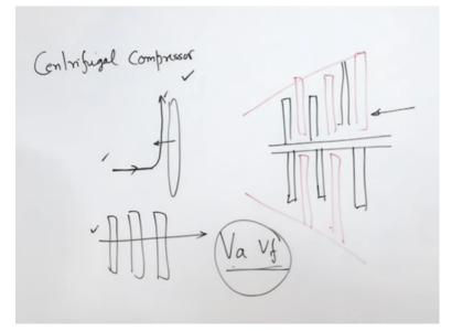
In centrifugal compressor, the fluid was entering along the shaft. There was an axial entry of the fluid or air and exit was radial. It was entering the compressor, there was an impeller, imparting energy or doing work on the incoming air and then air was compressed and finally, we got high pressure gas or air at the exit of the compressor. Now in axial flow compressor, the movement of the fluid is only in axial direction.
