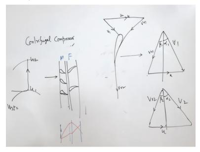
So each stage has fixed blade and the moving blades. Suppose there is a fixed blade like this and then there is small gap between these two and then there is a moving blade. So there number of fixed blades and there is a number of moving blades and they have mounted on the shaft, the shaft is parallel to this board and it rotates with a certain rotational speed. And the air moves in this direction axial flow direction.
