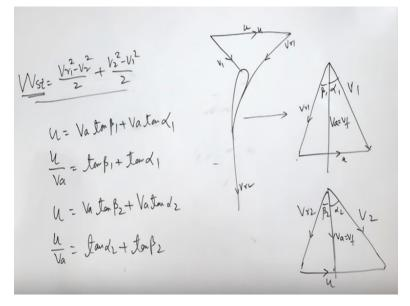
The work in a stage = VR1 square - VR2 square divide by 2 + V2 square - V1 square divide by 2, here peripheral velocity component is missing because there is nothing like U1 and U2. There is only one constant peripheral velocity so energy imparted to the fluid by virtue of changing peripheral velocity is 0. So if we look at this then per stage work in axial flow system we can say is less than the per stage work in centrifugal compressors.
