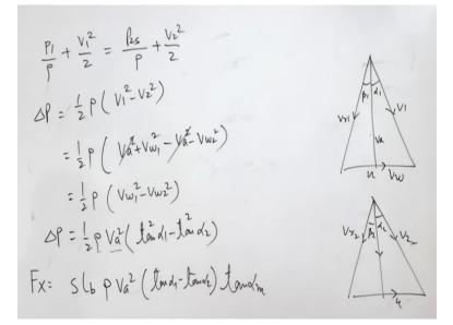
So we will start with Bernoulli's theorem, P1 by Rho = V1 square by 2 = P2 stage divided by Rho + V2 square by 2 because it is moving in horizontal direction prudentially production energy is 0. So Delta P is half Rho V1 square - V2 square Delta P.
