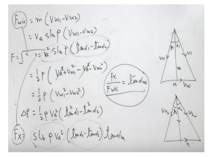
The willing force which is perpendicular to this one sorry this is an compressor, so compressor will have the force will be exerted in the axial direction force will also be exerted in willing direction and that force is mass flow rate multiplied by VW 1 - VW2 and that is V F S L N Rho. This is volume, this is density VW1 - VW2 and the net energy consumed by the axial flow compressor will be Pythagorean sum of this means net force.
