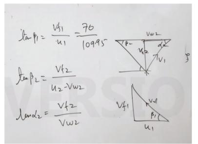
VF1 U1 VR1 and this is beta 1 so tan beta 1 = VF1 by U1 VF1 is 70 so it is 70 divided by 109.95 from here we will get the value of Beta1 is 32.4 degree right now similarly we will calculate now beta 2 is this is beta 2 right and this beta 2 is tan beta 2 is VF2 by U 2 - VW2 this is V1 and this is VW2 and this is VF2.
