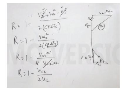
Why i have done this in a so suppose there will be a compressor for gas turbine this is VF and this is U1 and beta1 VF V1 ok so VF1 is V1 at the outlet this is VR2, U2, V2 right and this V2 = VF2 square or VR2 = VF2, VF2 square + VW two square now velocity of flow it is constant in this type of arrangement so this can be cancelled out and R = 1 – VW2 square divided by CP delta TS sorry.
