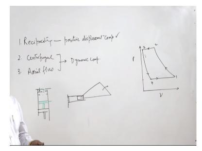
There are two types of compressors, one is reciprocating compressor, three types in fact reciprocating compressor they are known as positive displacement compressors. And another type is centrifugal compressors and third one is axial flow compressors and these are known as dynamic.
