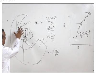
Instead of temperature entropy if you draw it is more the same thing if you draw enthalpy entropy or temperature entropy, enthalpy and entropy diagram for a centrifugal compressor. So initially the air is sucked in, so air is available at state 1, it is sunk into the compressor, so the pressure and the suction of the compressor is below the atmospheric pressure. Only then air can be sucked in and it is not an isentropic process.
