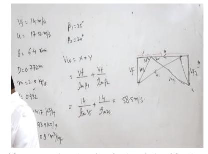
Now velocity of flow once we have the value of U the velocity of flow is 0.8 into 17.52 and this gives the velocity of flow as 14 metres per second this is the velocity of flow and now we have to calculate because we have to calc we have to find the power developed at this stage. So for calculating the power developed we need to have the value of VW will velocity.
