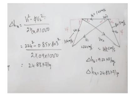
Enthalpy drop in blades enthalpy drop in the nozzle so enthalpy drop in the nozzles is going to be = V1 square 1, 5 V2 square by 2 nozzle efficiency into 1000 in order to convert rate into the kilo joules and that is V1 is 224 meter per second 10.85 multiplied by 80.3 square divided by 2 efficiency of the nozzle is .9 multiplied by 1000 and this will give the enthalpy drop in the nozzle is 24.83 kilo joules per kg.
