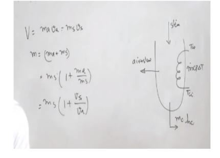
But volume of the shell is equal to mass on the air specific volume of the air is equal to mass of the steam. Specific volume of the steam right total mass in the vessel is mass of the air plus mass of the steam is equal to mass of the steam one plus mass of the air divided by mass of the steam is equal to mass of the steam one plus specific volume of the air mass of the steam mass of the air. So specific volume of steam by specific volume of air right.
