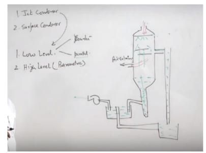
Jet condenser and another type is surface condenser but i was explaining to you was a is about surface condenser but in jet condenser mixing of cooling water with the steam takes place. So when the fresh water is available or clean is available are known as only this places are only those sides the jet condensers can be used now jet condensers are further classified low level jet condenser and number two is high level jet condenser or barometric jet condensers.
