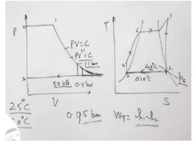
Which works on rankine cycle if i draw this steam power generation on Rankine cycle 1, 2 expansion 1 to 3 and 3 to 4 and 4 to 5. If you remember this diagram that 1 to 2 at state 2 the steam enters the condenser and the condensate is removed at state 3. Now for the steam power generations there are two devices one is steam turbine and another is steam engine.
