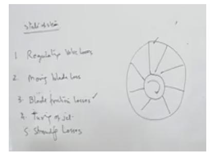
Shrouding losses in turbines is done. What is shrouding? Shrouding is suppose, if we look at the in view of the turbine I am just giving you the estimating view it is going to be like this. There are number of blades attached to the rotor and the rotor is moving with certain rotational speed. These blades are tied together with the help of shrouding and this shrouding also causes interruption in the flow.
