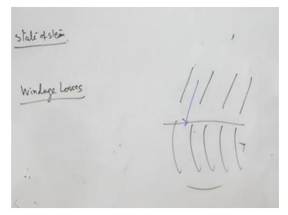
Another type of loss is windage loss now what happens is in high pressure turbine, especially in the high pressure area specially in the impulse turbine, there is limited number of nozzles and the limited number of nozzles all the blade passages are not directly exposed to the steam which is coming from the nozzle. In some of the blade there is partial admission.
