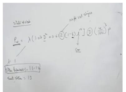
So in this case then again in P windage losses = lambda 1.07 D square + 0.610 Z 1 - epsilon L is to power 1.5 D U by 100 cube rho. It is difficult to remember but this is also an empirical relation where lambda from here is generalized equation. So for here it is one for super heated steam it is 1.1 to 1.2 and saturated steam = 1.3.
