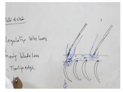
Second is moving blade loss, energy loss also takes place inside the nozzles. We will consider them later on, so now we will focus on moving blade loss. Now in moving blade loss first is let us take a nozzle and through this nozzle there are number of blade passages right. Nozzle has certain wall thickness right and steam is flowing in this direction and this wall does not exist in this alveolar space.
