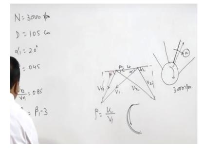
This is first numerical which states that for a single stage 3000 RPM impulse turbine. So there is an impulse turbine with RPM = 3000. The mean diameter of the blade is 105 centimeters. So the diameter is 105 centimeter.
