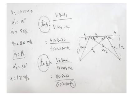
So here in this case V1 is given V1 is 400 meters per second and alpha 1 is also given is 15 degree. Steam at 5 kg per second, so mass flow rate is also given 5 kgs per second comes out of the equiangular moving blades with an absolute velocity of 80 meters per second. So V2 = 80 and equiangular, so beta 1 = beta 2. Nozzle outlet angle is 60 degrees so alpha 2 is also given 60 degree.
