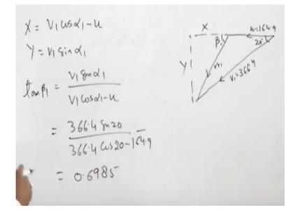
This is the value of U so in a velocity diagram we can always draw U and direction of U is this. Now blade inlet angle sorry this nozzle inlet angle is 20 degree. At 20 degree a line will be drawn and the length of this line is equivalent to V1, V1 is not given ok but we have the value of rho. Rho = U by V1 so V1 = rho by, so sorry, U by rho = U by rho.
