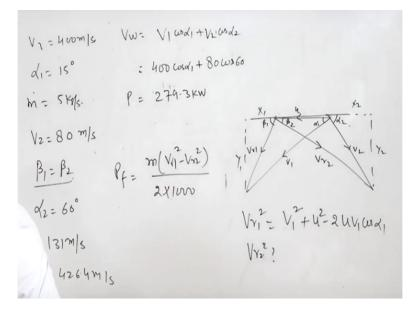
QF or power friction sorry power friction, mass flow rate VR1 square - VR2 square divided by 2 into 1000 right. Now we have the value of V1 we do not have the value of VR1.
