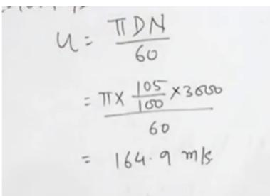
So U = PI D N over 60 we have taken because this is RPM. So this RPM is converted into rounds per second. So it is going to be PI into 105 divided by 100, converting into meter, into 3000 divided by 60 and U is going to be = 146.9 meters per second.
