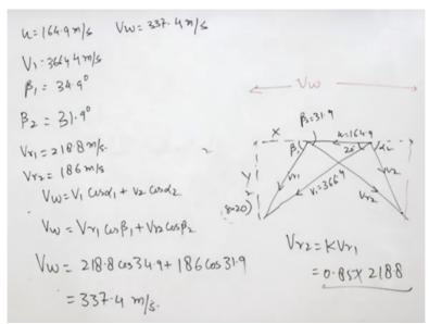
Now wheel velocity of the flow wheel velocity is this one this is wheel velocity right. Now wheel velocity can be expressed either like VW = V1 Cos alpha 1 + V2 Cos alpha 2. This is
