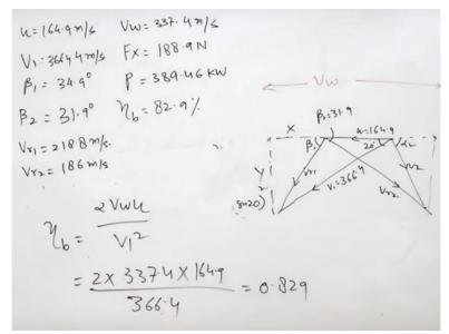
Now blade efficiency is 2 VW U by V1 square it is the blade or diagram efficiency. Now VW is with us so 2 into 337.4 into U, 164.9, divided by V1, we have it is given here 366.9, sorry 366.4 and this will give the blade or diagram efficiency 0.829 if you multiply this by 100, this is 82.9 %.
