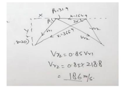
So VR1 is 218.8 meters per second but once we have the value of VR1 and this ratio the relative velocity at outlet from the blades to the inlet of the blades VR by VR1 is .85. So VR2 = 0.85 VR1 so VR2 = 0.85 multiplied by VR1 that is 218.8 and we will get the value of relative velocity at 2 is 186 meters per second right.
