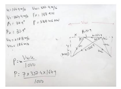
So power is VW U by 1000 this is the force multiplied by the velocity so and multiplied by mass flow rate. So VW is given so power is mass flow rate is seven, VW is 337.4 multiplied by U, peripheral velocity, we have calculated. 164.9 divided by 1000 okay and this gives the power as 389.4 kilo watt right so we are getting power also.
