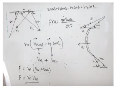
Because this is your channel with this turbine blade channel steam is entering like this blade velocity U in this direction and this is absolute velocity at inlet and this alpha 1 and this is
