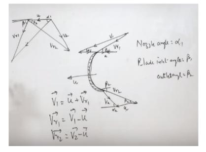
There is a suppose there is blade of an impulse turbine the blade NS i started earlier lecture the steam entering the blade should be such that the angle of entry the steam entering the blade should be such that the steam glides over the blade. Ok and this steam which is coming to the blade will definitely enter at a certain angle right and this angle is known as blade inlet angle right.
