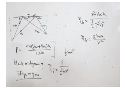
Output power is mass flow rate VW 1 + VW 2 or VW. VW 2 into U by 1000 that is one thing second thing is what is the efficiency of this blade there is a term which is known as blade or diagram efficiency blade or diagram efficiency either it is a blade or some others called blade efficiency or some others called diagram efficiency through this diagram the issue is we are getting this power output from this velocity diagram or the arrangement.
