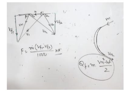
So when the steam is only gliding on the surface then this is VR1 and simply it is gliding on the surface and leaving from this side then VR2. So this velocity should not change so due to the fiction it is a change in this velocity in actual practice and this energy loss in fiction is MVR1 square - VR square divided by 2 this is kinetic energy the kinetic energy based on the relative velocity at inlet minus kinetic energy based on the relative velocity outlet.
