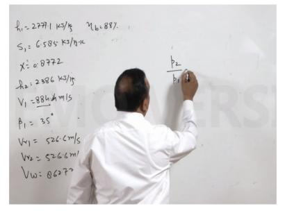
Or P2 by P1 is critical pressure ratio for steam expansion of a steam and that is = 2 by N + 1 is to power N by N - 1 = 0.577 right for a steam value is taken as 1.3 ok in that case we will get P2 = 577.4 kilo pa because P1 is 1000. So this is 5574 exit pressure is 100 kilo pa square it means it is a (()) (30:28) right.
