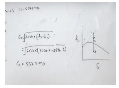
Now velocity state 2 C2 is going to be 2000 multiplied by H1 - H2 now I will rub this off H1 - H2 and under root. And this = under root 2000 multiplied by H1 is 3040.9 and H2 is 2896 and this will give the value of C2S 537.2 meter per second.
