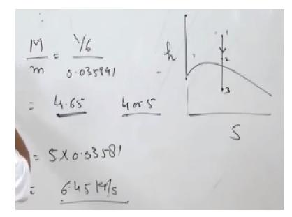
Per nozzle mass flow rate is this much so number of nozzles is going to be total mass flow rate divide by mass flow rate per nozzle total mass flow rate is 1 by 6 KG per second here is 0.035841 and that is going to be = 5.645 number of nozzle is 4.65 but we cannot have 4.65 nozzle. It has to be increase either 4 or 5 then we will have to take five nozzles.
