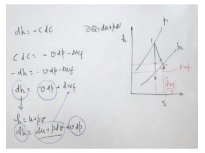
As we know that for the flow through a nozzle the change in enthalpy DH = -CDC change in kinetic energy and from momentum equation we have write that CDC = -VDP - WF. V is the specific volume W is the friction loss so if you compare this two equation that we get -DH = -VDP - WF or uses DWF right.
