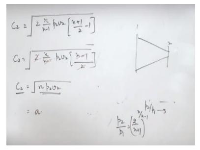
We can easily simplify this equation to find the value of C2 at the throughout C2 = now under root 2N upon N - 1 P2 V2 here this 1 - N, N - 1. So and this N and N will be cancelled out this is N - 1 this is 1 - N so this expression is going to be N + 1 by 2 - 1. Now C 2 is under root 1 N over N - 1 P2 V2 divide by 2 N - 1 now this N - 1 we will get cancel with this N - 1 this 2 will get will get cancel with this 2.
