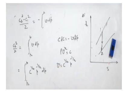
So as we know for the flow of the nozzles C2 square - C1 square by 2 = -2 to VDP. This we have derive from VDC = -VDP right C1 we can always neglect so C2 square by 2 = integral P2 2 P1 VDP. We always know that for polytrophic this is polytrophic process not his one expansion through nozzle.
