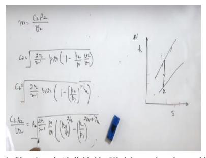
So mass flow rate is C2 at the exit A2 divided by V2 right now in order to achieve this what we can do we can take C2 = under root 2N upon N - 1 we can take out P1 V1 So we will be getting 1 - P2 by P1 multiplied by V2 by V1 fine now V2 by B1 = P1 by P2 power 1 by N or we can write P2 by P1 = P2 by P1 raise to power - 1 by N.
