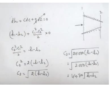
Let us take a passage or a of varying cross section the walls are rigid there is no walls on the movement of the muzzle fluid is flowing in this direction this is plain one this is inlet this is plain two at outlet and let us say this is control volume on which our study is focused very close to the wall right. And if we write first law equation for flow that is delta P by Rho + CDC by GDZ = 0 right or now this is DH.
