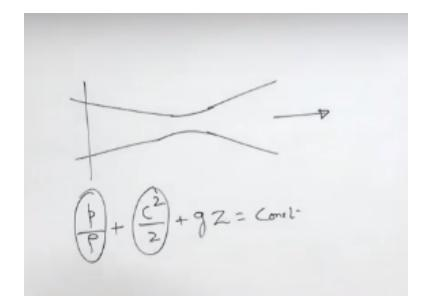
Nozzle is a passage of varying cross section it may be converging or diverging or the varying cross section may be converging and diverging as well. So it is a passage of varying cross section were pressure energy is converted into kinetic energy all of us know the equation T by rho + C square by 2 + GZ = constant. So in muzzle at the expanse of pressure energy kinetic energy is attained.
