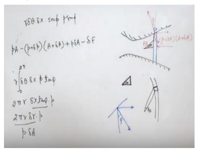
Because nozzle is a diverging passage this is a diverging passage and this angle is five. So when we take pressure from normal to for so pressure is normal to this surface so this angle is going to be 5 right. Now second thing is this is a ring of this vector ring around the periphery of the nozzle of thickness DX.
