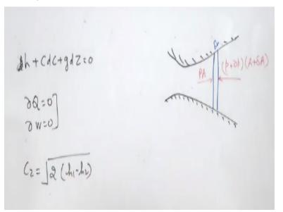
And let us take a thin section out of this of distance delta X now if you do the force balance on the section in this direction the force is pressure into area. Whatever pressure is exist on existing on this side multiplied by the area. Now existed on this from this side is P + Delta PA + delta A whatever it is because normally in the i mean in this direction there is a fallen pressure but to have a generalize equation we have taken P + Delta P existed on this direction right.
