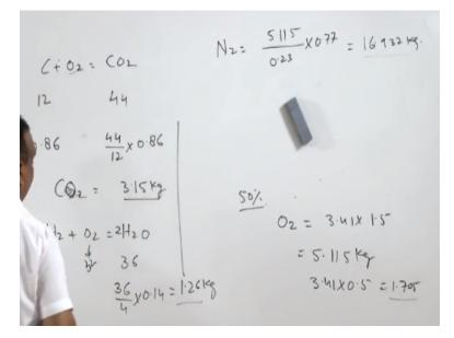
So when carbon dioxide carbon is oxidized to carbon dioxide C + O2 = CO2. So 1 KG of 1 mole means 12 KG of carbon 1 kilo mole 12 KG of carbon will form 44 KG of carbon dioxide right. So from this we have per KG we have 0.86 KG of carbon will form 44 by 12 multiplied by 0.86 and that will give 3.15 KG of carbon dioxide by mass.
