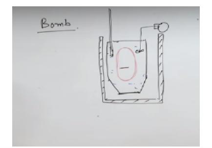
Now in order to find the calorific value of the fuel that the instrument which is known as bomb colorimeter Because finding out calorific value of fuel is also difficult task in bomb colorimeter I will just give you the schematic diagram there is a cylindrical vessel it is well insulated well insulated cylindrical vessel. Inside the vessel there is jacket sorry there is a bucket so bucket is placed inside the vessel and bucket is filled with the water, water I will show by different color.
