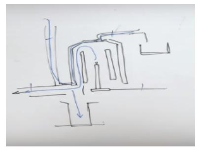
In a gas calorific meter there is a burner gas calorimeter in gas calorimeter there is a burner where gas is suppose burn gas supply is there it is house in a inverted vessel right an inverted vessel like this it is having water jacket this vessel is having water jacket and there is one water jacket here also right and water is supplied from this side and water is taken away from this side from the water jacket right and flue gases coming out of this they will go in this direction.
