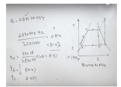
So Q in order to find the efficiency Q two 830.77 multiplies by 92 amount of steam produced by burning 1 KG of coal divide by 32 into 1000 and this will give the efficiency as 0.814 or 81.4 %. And the second term is heat absorbed by the heat water in various components as a % of total (()) (27:47) this is total heat and for individual component.
