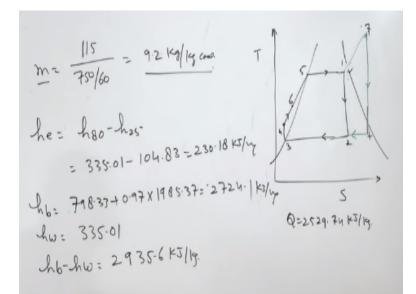
So steam produced here is a steam produced is 115 KG and that is KG per minute and coal is 1 KG per hour divided by 750 divided by 50 so that will give mass of the steam produced per KG of coal that is 9.2 KG per KG of coal. This is mass of the steam produced by burning per KG of coal heat added in economizer is H 80 - H 25 that is going to be = 335.01-104.83 and that = 230.18 kilo joules per KG.
