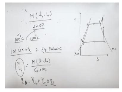
It means the mass of the steam produced is M then H G - HF that is the energy going with this steam. If you look at the rankine cycle then pressure and entropy then state one state two state three four and state 5. Heat edition in the rankine cycle takes place in state between the state four to state one the feed water goes to the boiler at state four and state one.
