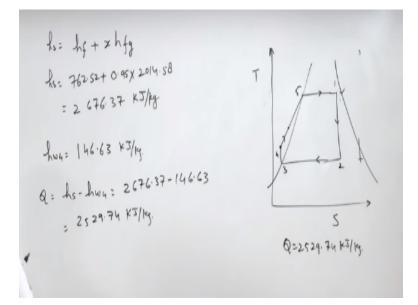
It means in a rankine cycle in this rankine cycle initially feed water was given at state four 35 degree centigrade then feed water was heated up to 100 degree centigrade in second condition so state is somewhere here and final state is remaining same right. So we will start with enthalpy of the steam enthalpy of the steam or enthalpy of the steam that enthalpy now here in this case the quality of the steam is .95 drive it will not be superheated.
