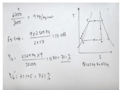
So steam generation rate is 6.3 tones per hour or 1600 KG per hour and coal consumption is .7 tones per hour .76 KG per hour. So per KG is burnt per KG of coal then we will be getting 9 KG of a steam per KG of coal. So equivalent evaporation is in this case is mass of the steam produced multiplies by energy spent in converting modern into the steam it is 25229.74 divided by 2257.
