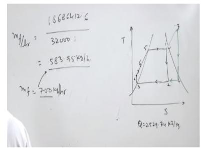
Now we will find mass of the fuel burned per hour right mass of the fuel burned per hour is heat supplied heat supplied is the simplification of this that is going to be 18686412.6 divided by calorific value of fuel that is 30,000 kilo joules per KG and that's it calorific value of fuel. So this is give the mass of the fuel is 583.95 five KG per hour.
