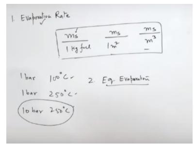
The number one is evaporation rate mass of the steam produce by the boiler divided by per KG of fuel or mass of the steam produced by the boiler per meter of heating surface area or mass of the steam produced by the boiler divided by volume of the grate that is also in meter cube. So either of these three we can express the evaporation rate but the evaporation rate problem with the evaporation rate is that.
