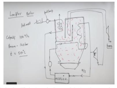
Am drawing with the simplified schematic diagram right there is a grate here the fuel is burnt okay a separate arrangement is made for steam generation it is separate from the boiler okay and here the generation of the steam takes place with the help of superheated steam. So first of all we will start with the hot well this is hot well consisting of water and as we did earlier also here the heat is extracted here will be extracted through an economizer by heating feed water.
