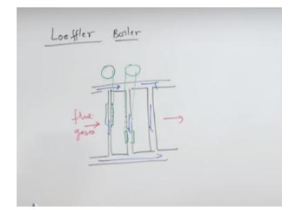
Will start with the Loeffler boiler now in this boiler we use turbines as well in this boiler not only there is a circulation of the steam turbines also that means that makes us interesting. Another feature of this boiler is that heat is generated with superheated steam. A steam it itself generated by superheated steam so there is a suit deposition in the evaporator.
