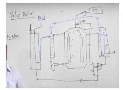
Again there is a sort of vessel in this vessel the fuel is supplied there is a fuel tank and from the fuel tank there is a feed pump and through the feed pump the fuel is supplied through this boiler this boiler is also supplied air at 3 bar pressure of the air is 3 bar. Now this air pumps this fuel and the velocity of the flue gases where even remain same because 3 bar schematic pressure is quite high pressure.
