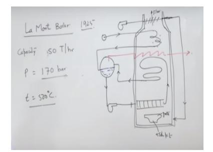
First of all it is a vertical boiler so the drum in the boiler is like this it is neck and passage for flue gases to go out from this passage flue gases leave the boiler right. Now at the bottom of the boiler the fuel is burnt and grate is provided lot of heat go out with the flue gases because I mentioned earlier the steam is generated 500 degree centigrade so definitely the heat carried away by the flue gases is relatively higher and with the help of air free heater we can tap this heat.
