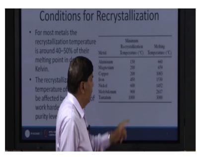
Since that recrystallization temperature for the brass is say around this what we have seen in the previous slide it is 200 degree centigrade so as soon as it is exposed very quick and rapid recrystallization takes place and this results in the significant drop in the strength of the brass as the exposure at high temperature takes place.
