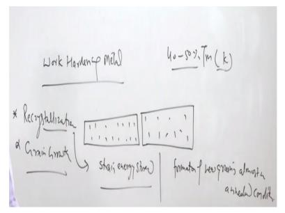
So we know that most of the metal systems during the manufacturing metal systems are deformed plastically and they get strength from that like the rolling or forging especially done under low temperature conditions. So under those conditions, plastic deformation will be developing lot of dislocations, which in turn will be increasing the strength and hardness of the metal system.
