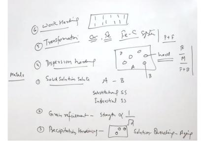
So we know that the different metal systems are strengthened using the different mechanisms and these includes solid solution strengthening where like in metal A solute B is incorporated so that the strength is achieved and the various types of solid solutions like substitutional and interstitial type of solid solutions are formed. Interstitial solid solution results in much higher strength with the addition of the solute as compared to the substitutional solid solution.
