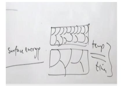
So driving force for the grain growth is the surface energy not the strain energy like the recrystallization and most of the metal systems made of large number of the grains, more number of the grains, large will be the grain bound area, more will be the grain bound area, great will be the surface energy related with that. So all metal systems try to attain the minimum energy for the maximum stability.
