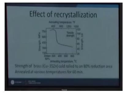
Say for this example, the material cold drawn up to 63% when it is given exposure to the higher temperature say 200 degree centigrade, there is no major drop in hardness, but as the exposure temperature is increased to 400, 600, 800 degree centigrade so there is a sudden drop in the strength of the brass, which has been cold drawn. This reduction in the strength takes place and this sharp reduction is attributed to the complete recrystallization, which is occurring for the brass.
