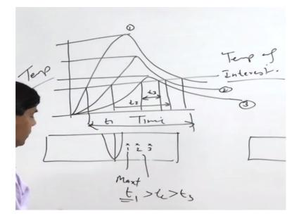
Further we know that whenever heat is applied obviously at the faying surfaces, fusion will be occurring and if we take the 3 points away from the fusion boundary then point 1, point 2 and point 3. We know that each point will be experiencing the different weld thermal cycle. One point will be experiencing the higher peak temperature and higher cooling rates.
