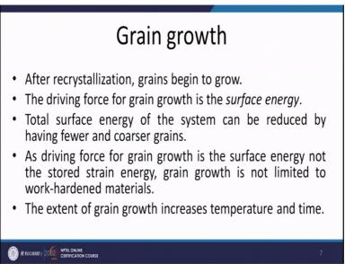
So grain growth will see now the way by which the grain growth is affected so this is what we can see. Driving force of the grain growth is the surface energy not the strain energy. So grain growth is not limited to the work hardened metal systems, but it is applicable in all the cases.
