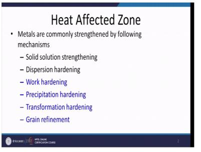
The solid solution is strengthened and the dispersion strengthened or hardened materials are somewhat less affected by the heat applied during the welding. While in case of the work hardening system, effect of work hardening is lost due to the annihilation or the recovery of the dislocations and the precipitation hardening due to the application of the heat during the welding heat affected zone near the fusion boundary.
