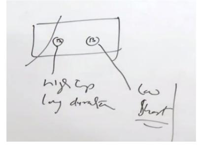
So the points close to the fusion boundary will have higher temperature like say A and B, A will have high temperature and long duration at high temperature as we have seen from the weld thermal cycle while the low temperature and short high temperature exposure so this is just opposite and this in turn will be reflecting in the weld thermal cycle so this is what the effect of weld thermal cycle.
