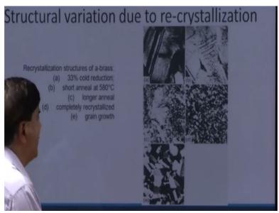
And whenever the heat is applied what you will see the material in very strained condition offers large number of the dislocations which we can see and when material is annealed for a short period, some of these dislocations are lost or these dislocations annihilate and further longer annealing results in the loss of this dislocations completely.
