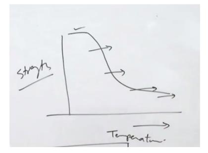
So which in turn will be lowering down the strength of the metal system say the temperature of exposure here if we have temperature of exposure as the temperature of exposure increases then the metal which is in work hardened conditions will be offering higher strength and as the temperature of exposure is increased will see there is a significant reduction in its strength of the metal system.
