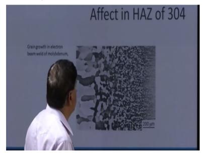
This is what we can see here the points which are very close to the fusion boundary will have the coarser grains and as we move away from the fusion boundary this will keep on decreasing the coarsening.
