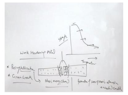
This is what we can see whenever the work hardening metal systems exposed to the external heat the metal systems near the heat affected zone recrystallize and formation of the new annealed grains lower down the strength of the metal as compared to that of the work hardened condition. So basically effect of the work hardening is lost due to the recrystallization.
