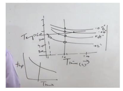
So this is what we can see here. In x axis we have time and in y axis is the temperature, so how the grain size like say this is for one, this is another and this is another like say if we consider 3 grain sizes, so for 0.02, 0.04 and 0.08 like this or we can have one more 0.06. This is in inches the grain size and typically the temperature values from 300, 400, 500, likewise and the time in log scale 1, 10, 100, 1000 like this.
