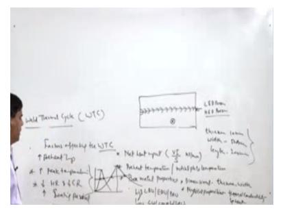
If this point is located away from, then we will see that, what we will see, with the increase in preheat, what we get, simply increase in the heat temperature what it does increases the peak temperature, if it is located away from one but at the same time it reduces the heating rate and it reduces the cooling rate. So these are the two things at the same time it will be increasing the soaking period.
