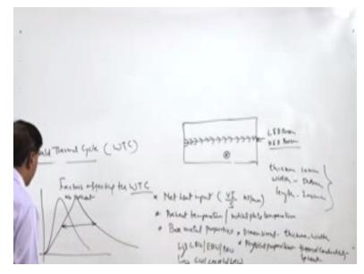
Another point is about the preheat temperature, so in case there is no preheating, the things are at room temperature, so the things will go like this, means the rate of heating is high and the rate of cooling is also high when there is no preheat and say and when the preheating is used the rate of a temperature rise, decreases, it reaches to the peak temperature and then it is starts cooling slowly.
