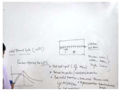
Like say here the point is this one and for this point if we will see weld thermal cycle in case when this weld is made using both low energy density process and high energy density process. High-energy density processes like laser beam so, what kind of her the thermal cycle we will getting in case of low-energy density process, will be getting higher peak temperature and then lower cooling rates.
