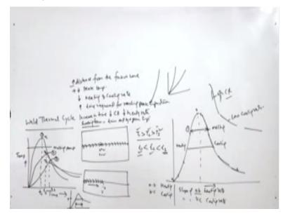
So the topic is weld thermal cycle, weather it is the fusion welding or the resistance welding whenever the external heat is supplied for the purpose of the softening of the metal like say infusion welding, the weld is made like this by applying the heat through arc or through the flame and if we see the different points, either in the weld central line like location 1 or slightly away from the weld location 2, location 3.
