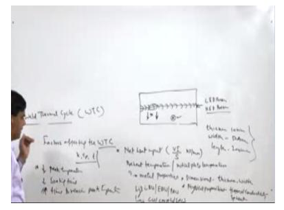
This is what we can mention for this purpose that the increasing thickness, increasing thermal conductivity for a particular point lowers the peak temperature, it reduces the soaking time above a particular temperature of that point like say the point is here so with the increase in thermal conductivity specific or the thickness of for this particular point the peak temperature will be reduced, soaking time will be reduced.
