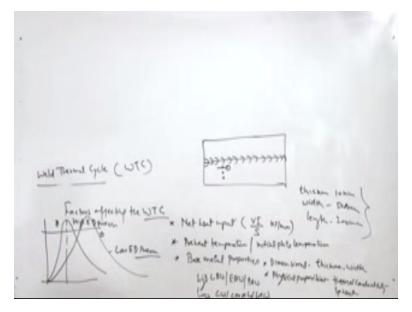
So when the heat input is low, in that case we supply very less heat to achieve the fusion or the melting of the base metal and in case of the high heat input we need to do a lot of heat for achieving the fusion. So in both the cases, in case of high heat input, the rate of the heating is so, in case of the low heat input for high energy density processes. It goes like this and for another low-energy density processes, it will be going like this.
