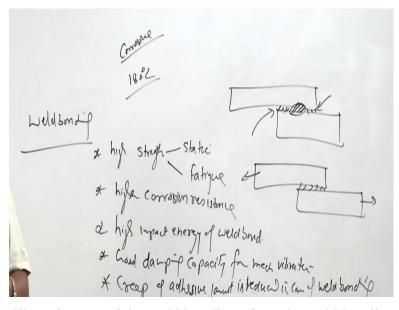
So here what we will see in case of the weld bonding, since the weld bonding is combination of the two processes so it overcomes the deficiencies of both the processes and provides much better strength to the joint so the - the weld bonding offers much higher strength - strength both static like tensile shear load carrying capacity or the dynamic or fatigue, so fatigue strength of the of the weld bond is found to be much higher than the spot welds.
