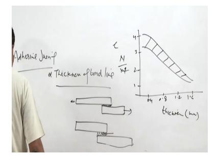
So as far as - as far as this one is concerned we will see the factors associated with the adhesive joining - adhesive joining first is say thickness of bond line or thickness of the adhesives, so what we can see here like this shear strength in newton per - shear strength in newton per meter square like say 1, 2, 3, 4 like this and the thickness of the adhesives in mm like say here 0.4, 0.8, 1.2, 1.6 in mm.
