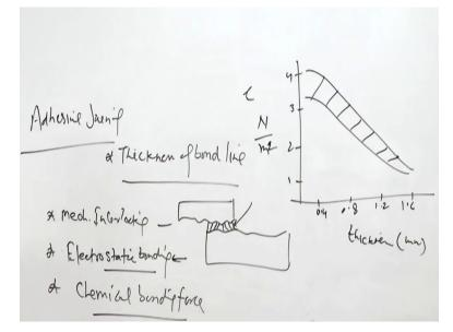
One is mechanical interlocking, two is the electrostatic bonding, three is the chemical bonding forces, so mechanical interlocking basically all the services have the regularities peaks and valleys at the surface when adhesive is applied it fills in the peaks and valleys of the - of the surfaces and thereby it provides the mechanical interlocking.
