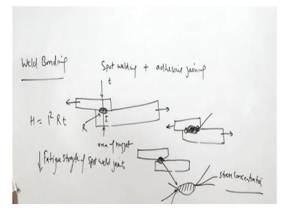
We know the typically spot welds - spot welding is used for producing the lap joints like this by supplying the high current through the contact interfaces high contact resistance at the interface develops heat and this is how pressure is applied and current flows through the interface current I is allowed to flow for the time t and contact resistance at the interface R helps to develop the heat through I square R t heating.
