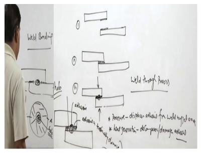
While in case of the weld through process in this case the first the adhesive is applied at the faying surfaces like this usually and then they are brought together like this, so here we have the plates in lap joint configuration with the adhesive, so the first step adhesive is applied then they are brought together in third step we develop the spot weld like this so when for during the spot welding when pressure is applied current flows it results in the two things.
