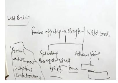
So as far as factors affecting the - factors affecting the strength of the weld bond we need to see both the processes. there are two processes, one is like say spot welding and another adhesive joining, so accordingly there will be factors associated with the both processes so strength of the spot weld is affected by basically the nugget area of - area of nugget of the spot weld and which in turn is governed by the kind of heat being generated which is I square R t.
