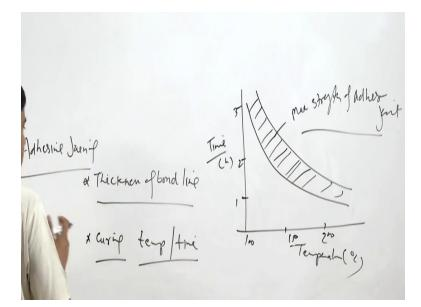
Second one is the - the curing aspect which includes the temperature as well as time, so if we will see the combination of the time and temperature for the curing in y axis if we have time in hours and in x-axis we have temperature in degree centigrade then what we will have like say 100 degree, 200 degree, 300 degree, I say 150 and 200 degree centigrade and in y axis we have 1, 2 and 3 hours.
