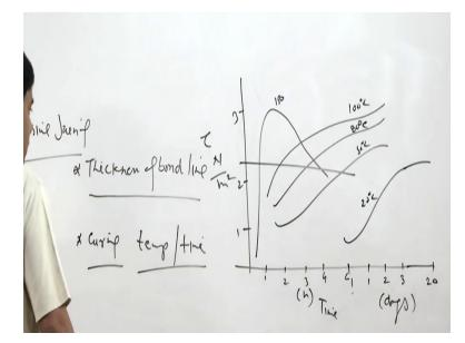
So now we will see one more diagram where we will be seeing the effect of the curing time and temperature on the shear strength of the joint, so shear strength of the joint in newton per meter square we will see here in y axis if we have time we will be using two scales basically just to show very long period of the time of the curing so here say it is 1, 2, 3 hours 4, 6 and then say 1, 2, 3 and here say 20.
