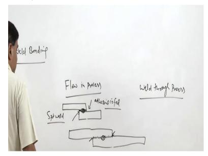
And the name of these approaches is like flow in process and another is weld through process, the basically the difference is in that it in which stage the adhesive is applied between the faying surfaces. so in flow in process what we do first the plates are taken or sheets are taken they are put in faying in the required configuration and then spot weld is made, so first the spot weld is made.
