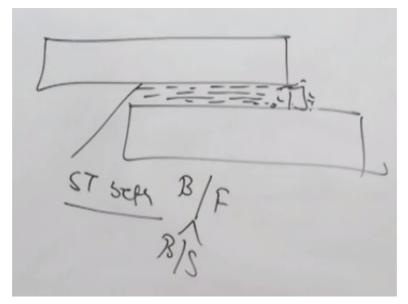
Then, once the solder is placed like say during the operation how does it work, like say this is the solder, flux is also applied so basically all will be reaching to the molten state here, the flux will also melt, solder will also melt. So depending upon the surface tension between the base metal and flux and base metal and solder, so the surface tension between the base metal and the flux being lesser than that between the solder.
