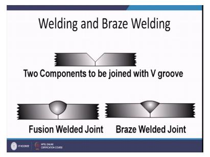
This is what I have explained like initially if the edges are prepared like this for developing the joint in case of the fusion weld, the faying surfaces are melted and we get the typically curved geometry of the fusion boundary. Well, in this case there is no fusion of the faying surfaces so the faying surfaces remain straight, the edges remains straight, only the gap is filled in by the brazing material. So this how we can easily distinguish between the fusion welds and the braze welds.
