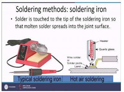
So here will see the two methods like soldering method using soldering iron is the typical soldering iron. So here it is very low capacity kind of the heating arrangement where once the
