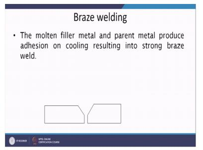
So melting of the faying surfaces hardly takes place and the molten filler metal and the parent metal produce the joint by adhesion on cooling result in the strong braze weld.
