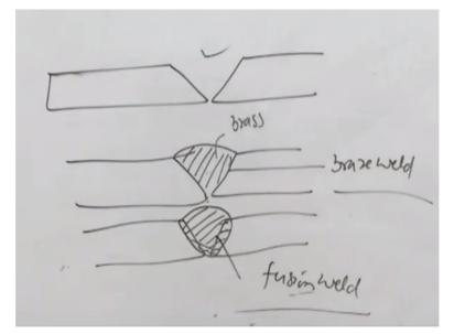
Then we have to see on simple diagram, which will clearly indicate that if this is how the plates have been prepared for developing the joint, in case of the braze welding, the surface of the base metal remains intact and rest of the gap is filled in by the brass. While in case of the welding, the faying surfaces melt and the geometry of the edges of the plates gets modified like this.
