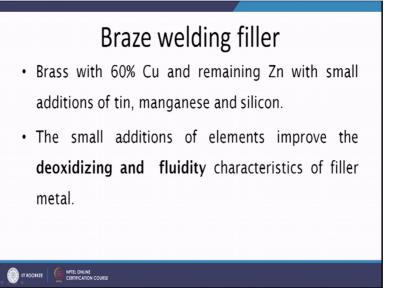
The brazing filler mostly 60% copper, it is a brass with the remaining zinc amount while small amount of the other alloying elements like tin, manganese and silicon are added for achieving the specific functions like deoxidization and improving the fluidity of the filler so that it spreads in course of the braze welding process and it occupies the different gaps whatever ups and downs expertise peaks and valleys are present on the surface of the material.
