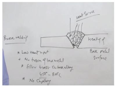
Here the principle of the braze welding is like this wherein the components to be joined are first prepared for the surfaces, so a groove is made between the components to be joined. Of course all those benefits related with the braze welding whatever were available for the brazing are also available in the braze welding.
