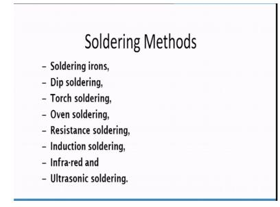
So depending upon the heating method like soldering iron, dip soldering, torch soldering, oven soldering, resistance soldering, induction soldering, infra-red and ultrasonic soldering. So these methods primarily differ in the way by which the heat is applied to the base metal and the way by which solder is placed or applied between the faying surfaces to be joined.
