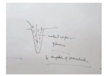
So this is what is obtained in key hole approach, but it imposes certain problems like high energy density results in the evaporation of the metal and a metal vapours, actually ionised, an ionisation of the metal vapours forms the plasma and this plasma absorbs the laser. So whenever plasma is formed in this gap the plasma absorbs the last and which in turn reduces the actual energy being delivered at to the base metal and that in turn reduces the depth of penetration.
