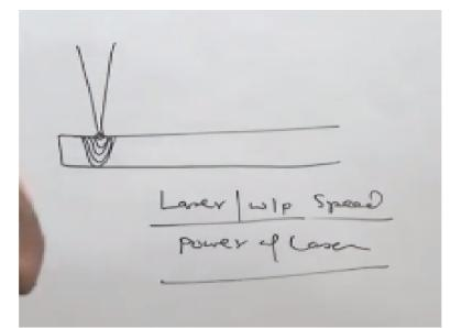
So you see melting will be taking place like this. So if it keeps on increasing the duration of this state, the depth penetration will keep on increasing up to certain limits. So we have to
