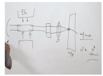
In this one basically the most common way is to that the lamps mainly called flash lamps are used to excide the material mostly in the form of ruby crystal and from this after the excitation the laser radiations are emitted like this, then they are reflected back using suitable reflectors. Here like this and then they are brought to the parallel then through the lines it is focussed at the desired point and this point becomes the workpiece.
