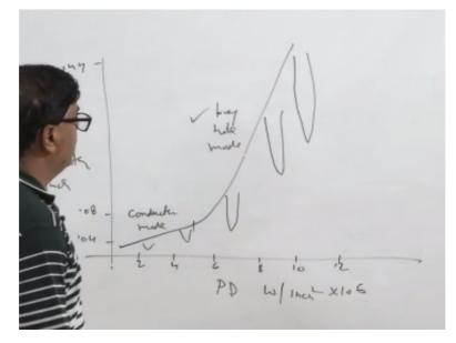
So for this purpose, what we need to see is one diagram, here we have power density in terms of the watt per square inch in 10 to the power 6. Here like say 2, 4, 6, 8, 10, 12 like this and on the other hand, the penetration depth which is achieved in inches it is like 0.4, 0.8 and like this 0.44. So when the power density is increased what we get like initially it keeps on increasing linearly like this and then it jumps fast.
