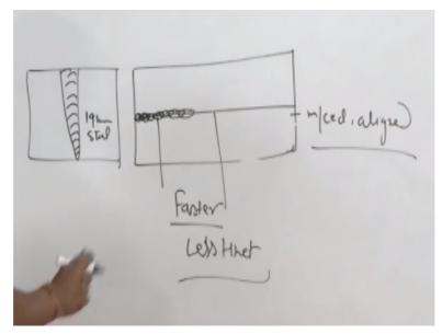
So amount of heat actually required for the welding purpose or for fusion purpose is very small. So here you see these are the two sheets to be welded and the two sheets to be welded must be properly machined aligned. This is very important in case of laser accurately machined and aligned if any gap is left between the 2 plates to be joined, like see the gap is if say 300 micrometer between the plates due to the machining accuracy or misalignment.
