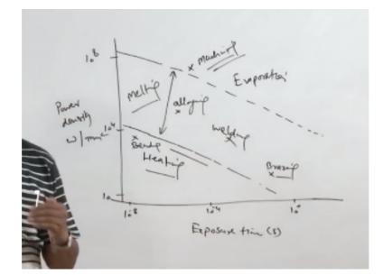
So there is one very general guideline kind of the diagram, which will help us to see the kind of approach, which is used. Here in the x axis we have the exposure times means the time for which the laser is applied. So here extremely a small say -10, 100 - 10, 10 to the power -4 and 10 to the power 0 and in the y axis, we have power density or energy density, which is in watt per mm square.
