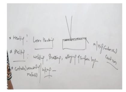
So by regulating the energy density we are in position to use it for the heating purpose, which is basically used for the like say laser hardening material is heated rapidly at the surface and then by auto-quenching or by external quenching it can be harden like say, the surface is directed with the laser and here it gets heated, reaches to the rising temperature and then it is quenched off as laser moves away from the directed surface.
