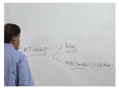
With respect to the cold metal transfer welding, it incorporates the two aspects. One is the pulsing means the pulse feature and another is efforts are made to regulate the metal transfer in a very controlled way through short circuiting mode. So, these two things are clubbed in case of the cold metal transfer welding. How it is realized for this using the electronics and the controlled movement of the electrode what is done in this case?
