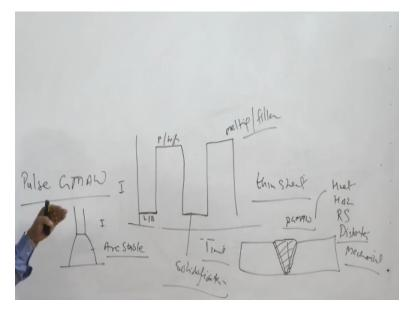
So to avoid that the GMAW process is modified in a particular way where in the value of current is regulated as a function of time. So, what is done in case like here we have current and the current value initially we will keep the current value less like say this is the welding current, also this welding arc and current is fed. So, the value of current is regulated. The first like say the low level of current or you can say background current like this.
