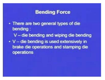
So, now, we come on to the bending force. We require some force to change the shape of the sheet or in order to bend the sheet according to our desired level or desired specifications. So, there are two types of die bending. So, the force depends upon the die bending. So, V bending and wiping die bending. So, there are two types of die bending processed are possible: first one is the V die bending and second one is the wiping die bending.
