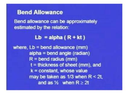
Now, we have seen that there are number of parameters. So, bend allowance is one of the parameters. So, bend allowance can be approximated by the relation. So, a mathematical relation is given for the bend allowance. So, bend allowance basically is given by Lb. It is given depicted by Lb or designated by Lb which is equal to alpha times the summation of R plus kt.
