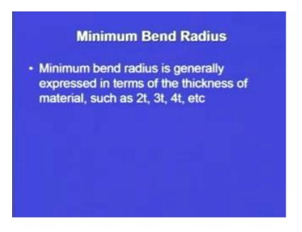
So, that is bend radius whenever we have to specify, we will specify in terms of thickness of the sheet. So, this thickness of the sheet can be for example, we can say 2t, 3t, 4t 5t. So, depending upon this particular value, we can say that what is going to be the minimum bend radius for that particular material.
