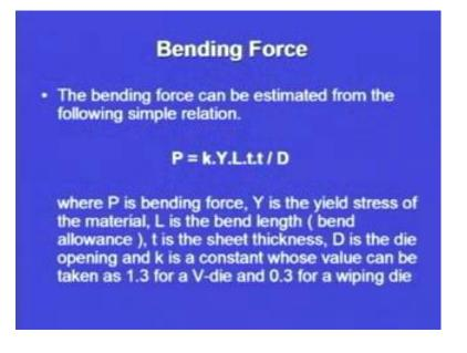
So, minimum bend radius already we have seen; it has to be specified and it depends upon the material there for which we are going to form the bend or of which the sheet is basically made of. So, this force required for bending is given by this equation. The bending force can be estimated from the following simple relation.
