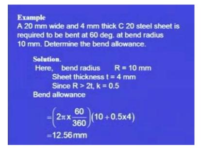
So, now we take an example. The example states this is the problem; it is a numerical problem; we can solve it and we can see that how the bend allowance can be calculated. The mathematical formula we have seen in the previous slide. How that formula can be used to calculate the bend allowance that will be seen in this example. So, the problem states that at 20 millimeter wide and 4 millimeter thick C 20 steel sheet.
