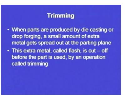
Then another important sheet metal operation is the trimming operation. So, in trimming, when parts are produced by die casting or drop forging, already we have seen what is a drop forging or we can make any product by die casting. So, whenever a product has been made using the die casting operation or it has been made using a drop forging operation, a small amount of metal gets spread out at the parting plane.
