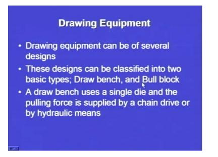
Now, we have seen that drawing equipment is required to reduce the cross section from a larger to a smaller cross section. So, if a wire or a solid wire is being is has to be reduced from a larger cross section to a smaller cross section or a tube has to be drawn from a larger cross section to a smaller cross section, we have to make use of a drawing equipment. So, drawing equipment can be of several designs.
