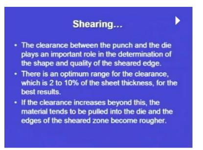
The clearance between the punch and the die plays an important role in the determination of shape and the quality of the sheared edge as already has been addressed. There is an optimum range for the clearance. So, there is an optimum range that has been decided depending upon certain experimental findings. Some research work that has been done in this field of shearing of sheet metals, that there is an optimum range that varies from 2 to 10 percent of the sheet thickness.
