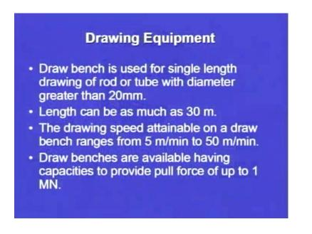
Now, a draw bench is used for a single length drawing of rod or a tube with diameter greater than 20 millimeter. So, there is a limitation on the diameter, if the diameter is greater than 20 millimeter we can use a draw bench, and it has single length drawing process. So, single length drawing of rod or tube is done, and the diameter should be
