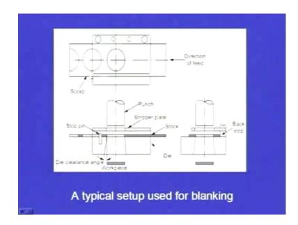
Now, this is the typical setup for blanking operation. We can see that this is the direction of it this is what is the scrap? This is the sheet that is being fed as the raw material. So, this is the scrap only this portion that is getting removed, this is the portion that is getting removed. This is the top view, if you see this view from here we can see this is the punch, the punch is here. This is the axis as has been shown see, the cursor is moving along the axis.
