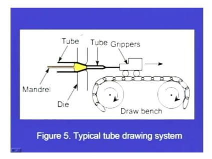
Now, here we see, this is the basic diagram of tube drawing very simple diagram, just to see what how the diagram has been labeled. We can see there is a mandrel as already discussed in the basic definition of wire drawing or tube drawing. That in tube drawing we make use of a mandrel, this is the mandrel we can see this is yellow color mandrel. Now, this is the tube the black color, the solid black section that is being drawn here. So, the tube is being drawn a mandrel, it is being used.
