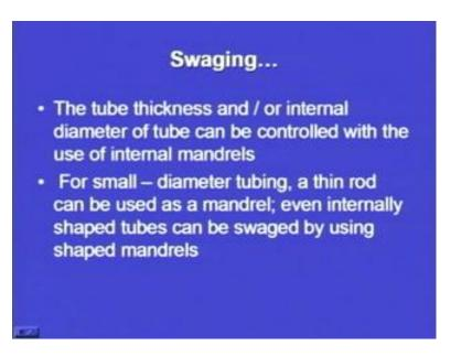
Now, coming on to the basic principles of swaging, the tube thickness and or internal diameter of tube can be controlled with the use of internal mandrels. So, now when we want to control the internal diameter or we want to control the thickness of the tube, we can use the mandrels. So, these mandrels can be of different shapes, suppose we want to
