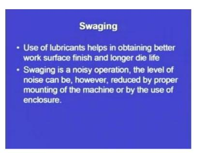
Another important aspect is the use of lubricants. So, why lubricants are required, wherever we are using a die arrangement, the die needs a lubricant otherwise the wear will reduce the life of the die. Moreover the surface finish of the product that we will get will not be up to the desired level. So, use of lubricants help in obtaining better work surface finish and longer die life, so already this has been discussed.
