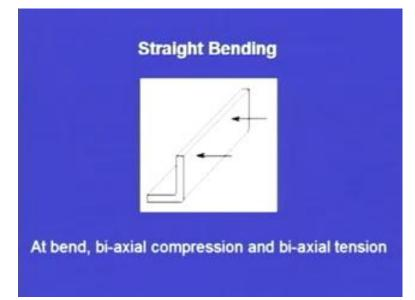
Now, in case of straight bending the straight bending we can see the load is applied, the arrows show in the direction in which the load is applied. So, at the bend, bi axial compression and bi axial tension are present. So, we have seen different types of metal forming operations starting from rolling, forging, then we have seen different types of deep drawing operations, tube drawing, wire drawing, state bending.
